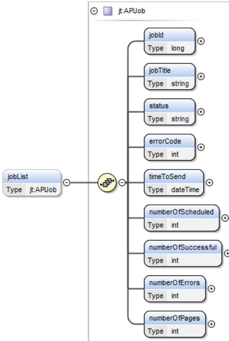
A UML class diagram showing a jt:APIJob object with several properties. The properties are listed in a vertical stack: jobId (Type long), jobTitle (Type string), status (Type string), errorCode (Type int), timeToSend (Type dateTime), numberOfScheduled (Type int), numberOfRowsSuccessful (Type int), numberOfRowsErrors (Type int), and numberOfRowsPages (Type int). Each property is represented by a blue rounded rectangle with a plus sign. |
